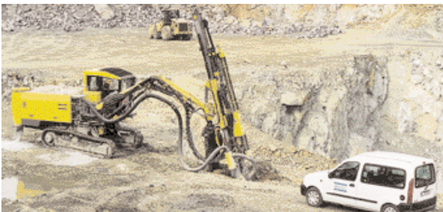
Newcomer to the site: The ROC D7-11 surface crawler rig has halved the cost of drilling and cut the consumption of bits, shanks and rods.
