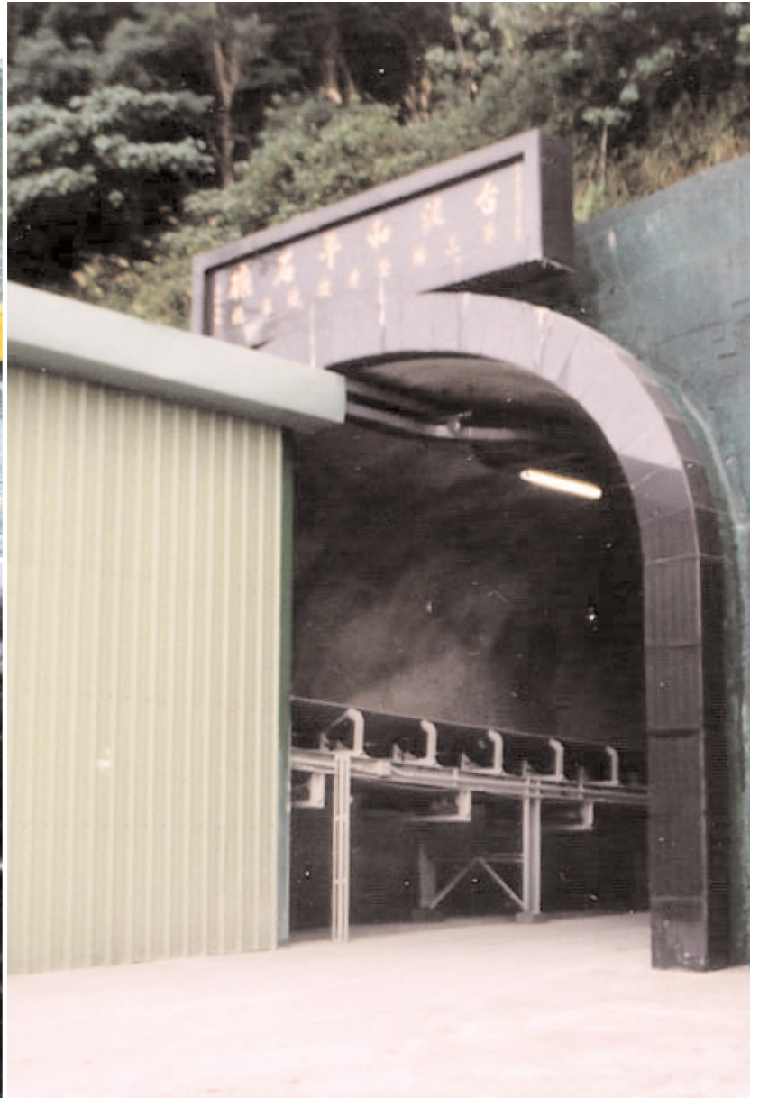
Hilltop challenge: The drillers at Ho Ping quarry, the largest limestone operation in Taiwan, use Atlas Copco ROC crawlers – including the ROC F9 with Coprod – to drill 127 mm holes up to 30 metres deep. To reduce noise and truck movements, the limestone is tipped down a shaft and transported out via a system of tunnels equipped with conveyors.
