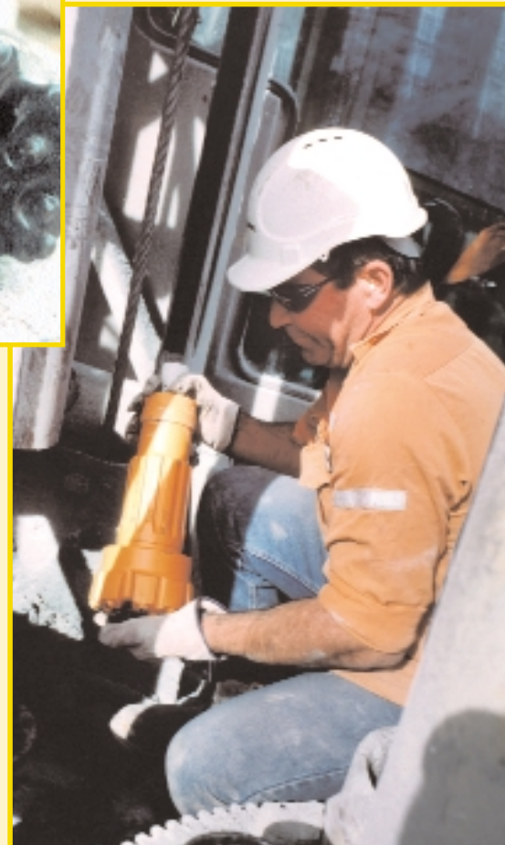
Ready for drilling at Super Pit: A new DTH drill bit, featuring 18 mm buttons and a 12 spline shank design.
