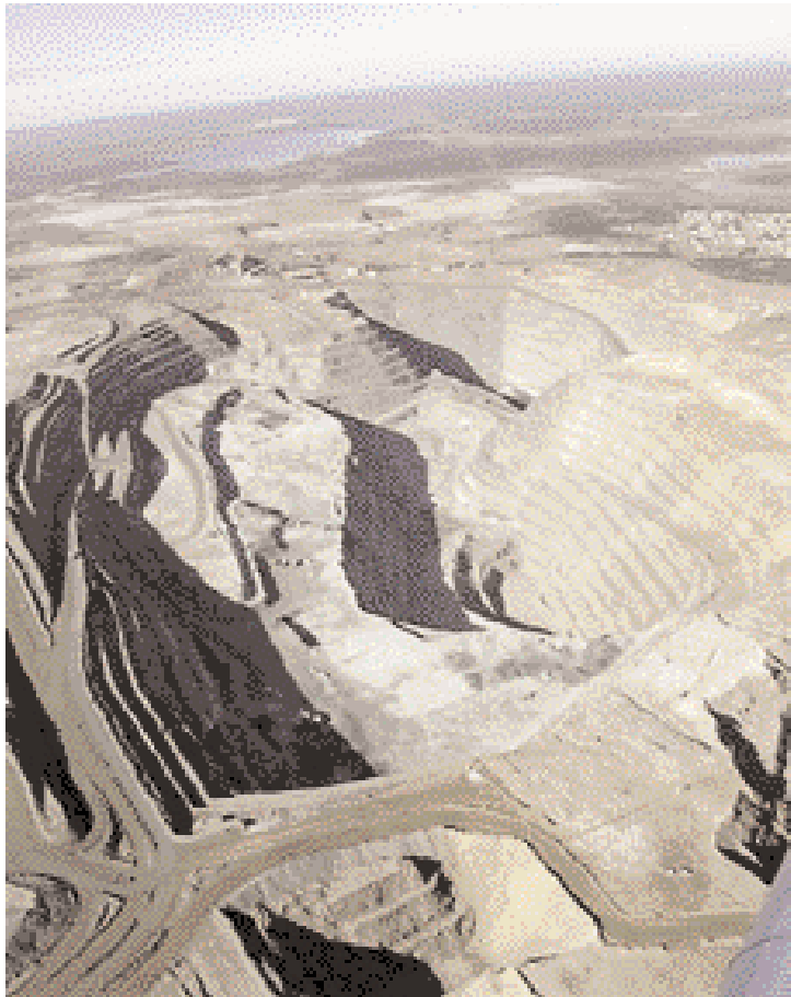
Located on the richest square mile of gold bearing ore ever discovered, the Super Pit is 290 m deep, 3 km long and 1.5 km wide. In the next decade it is expected that mining will be conducted 600 metres below the surface.
