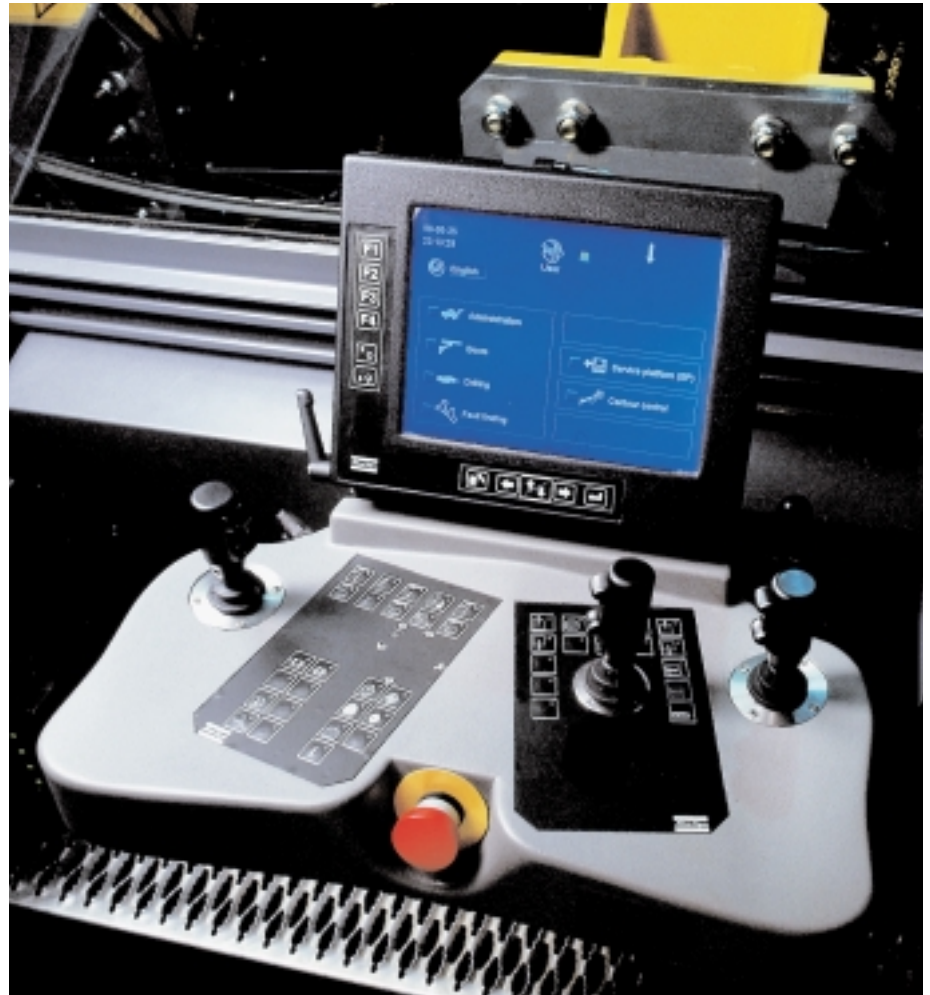
The workplace of today: The rig operator can simply supervise while the screen informs him of every phase of operations that the Rig Control System is carrying out.
